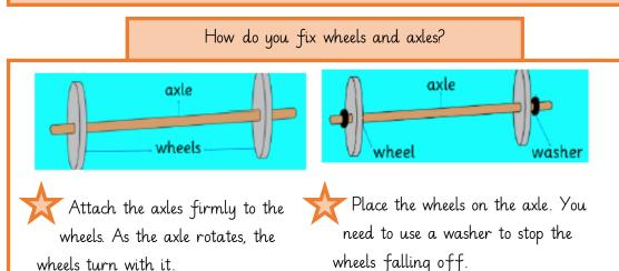
Attach the axles to the underneath of the chassis. The axles will not turn. Attach the wheels to the axles firmly so that they can rotate around it.
