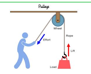
Pulleys are a simple piece of engineering which allows you to lift objects up and down using a cable or rope. They're made up of a wheel on an axle that rotates, allowing the rope or cable to feed around the groove within the wheel.
